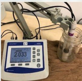
**FIGURE 1.** EC meter probe soaking in standard solutions.
